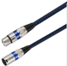
K7066CD-BLB 3P XLR Female To 3P XLR Male Metal Shell Mic Cable Double Shielded 60% OD:6mm Black Soft Cable + Blue/Black Polyester Sleeve
